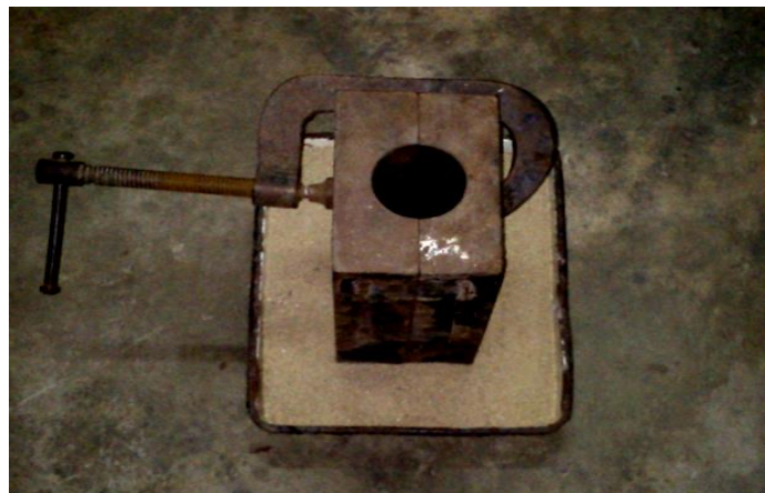
Figure 4.1) Die used for Composite preparation
